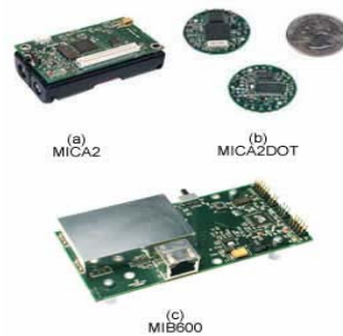
Figure 2 Wireless sensor network, including base station that provides the receiver-to-Ethernet link, at bottom ( www.xbow.com )
